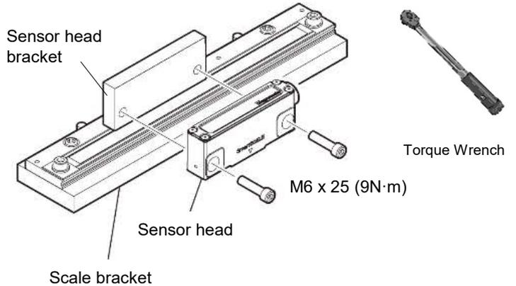
Insert the SZ26 between the sensor head and the scale. Then fix the sensor head under condition of light contact at both ends.
