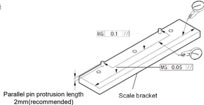
If the effective length is 1000 mm or less, Two  $\phi$  6 mm pins (38 mm from both ends of the scale) are recommended
