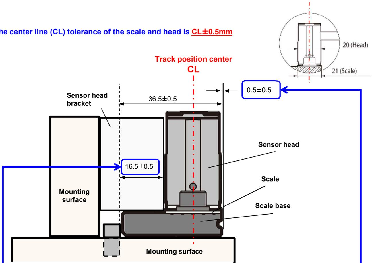
When mounting the actual scale, you can check the track position of the sensor head with respect to the scale if there is a space where a jig can be used either on the front side or the back side of the scale.
