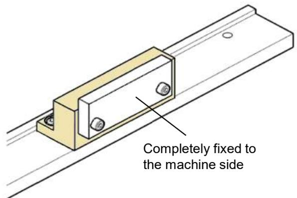
**Step ⑤: Removal of positioning jig**
