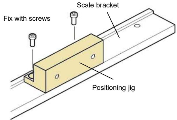
**Step ③: Installation of head bracket**
