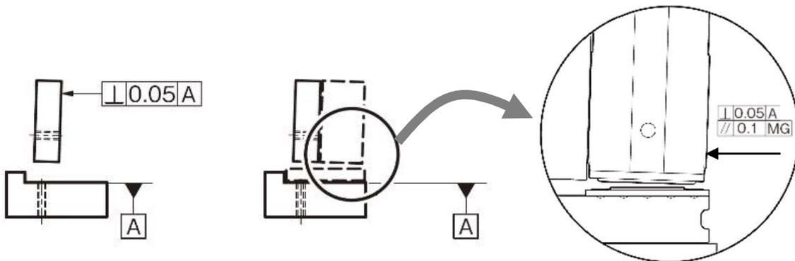
**Sensor head mounting tolerance to the scale surface**
