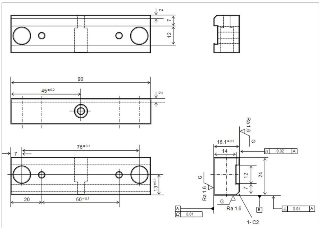
Note 1: No burrs on each surface, chamfering of unspecified corners is C0.5 or less
