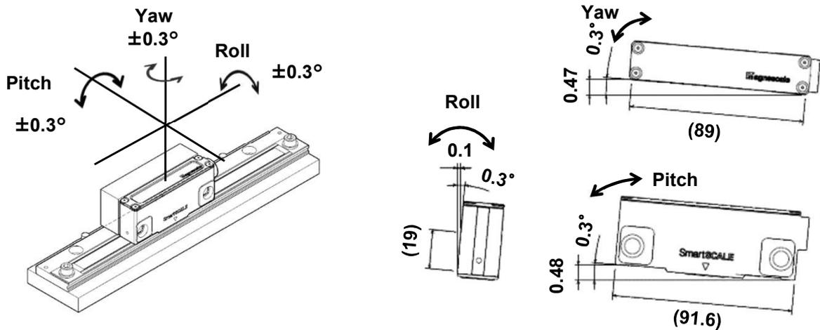
**Step⑥: Mount the sensor head (Clearance and pitch adjustment)**
