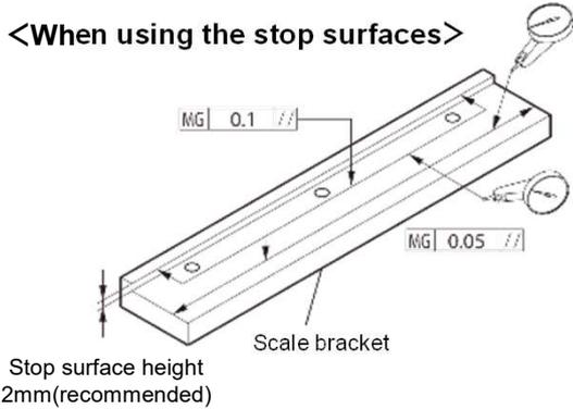
**Step ②: Fix the positioning jig**
