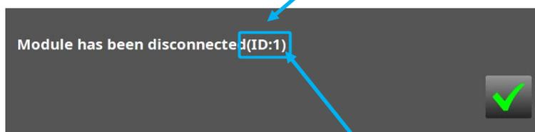
Displays the ID of the module with which communication has been lost
