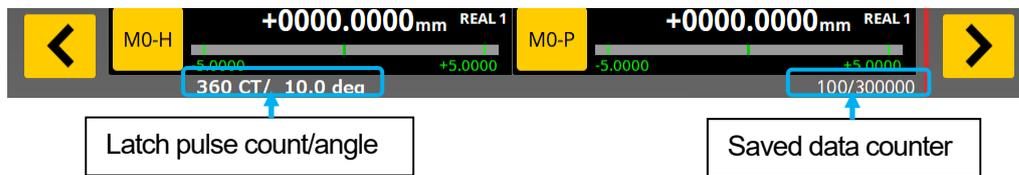
\* The saved data counter displays the number of data saved in the display unit. The maximum number of saved data is 300,000 data.
