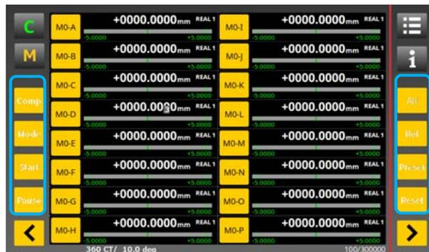
The current position of the encoder and the number of data acquired are displayed at the bottom of the measuring screen.
