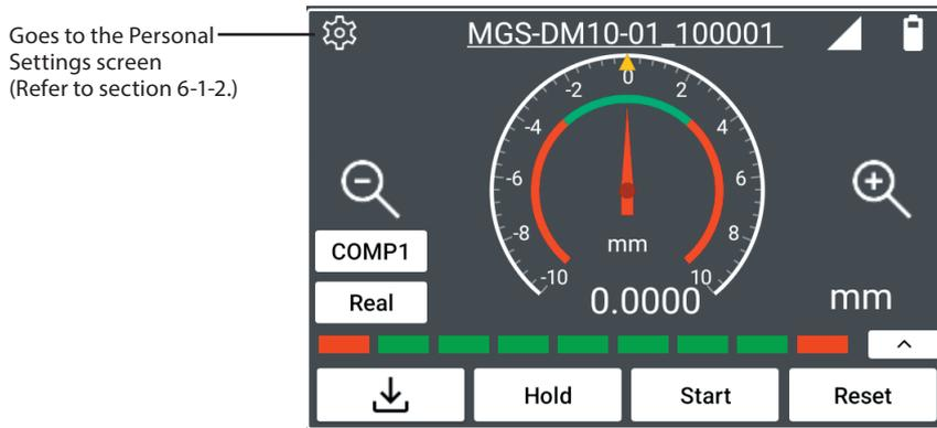
The contents for the connected measuring device are displayed. For details of each item, refer to the operation manual of the measuring device.
