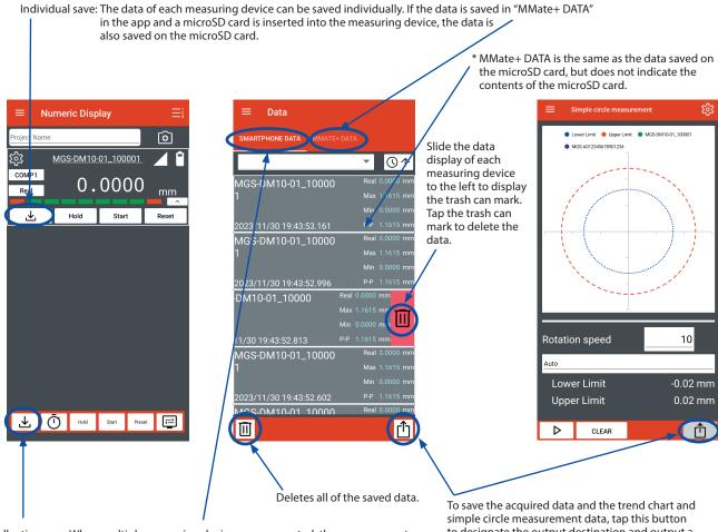
Collective save: When multiple measuring devices are connected, the measurement values of all the measuring devices can be saved simultaneously. The data is saved in "SMARTPHONE DATA" of "Data" in the app. The data is not saved on the microSD card of each measuring device. to designate the output destination and output a CSV format file.
