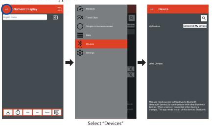
**4** Tap the magnifying glass tool " \( \sqrt{} \)". The measuring devices available for connection are displayed in "Other Devices".
