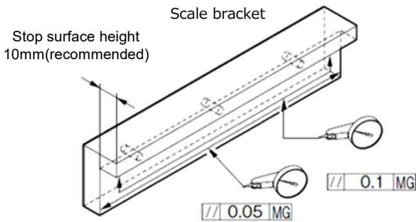
**Step ②: Fix the positioning jig**
