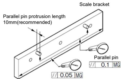
If the effective length is 1000 mm or less, Two  $\phi$  6 mm pins (38 mm from both ends of the scale) are recommended
