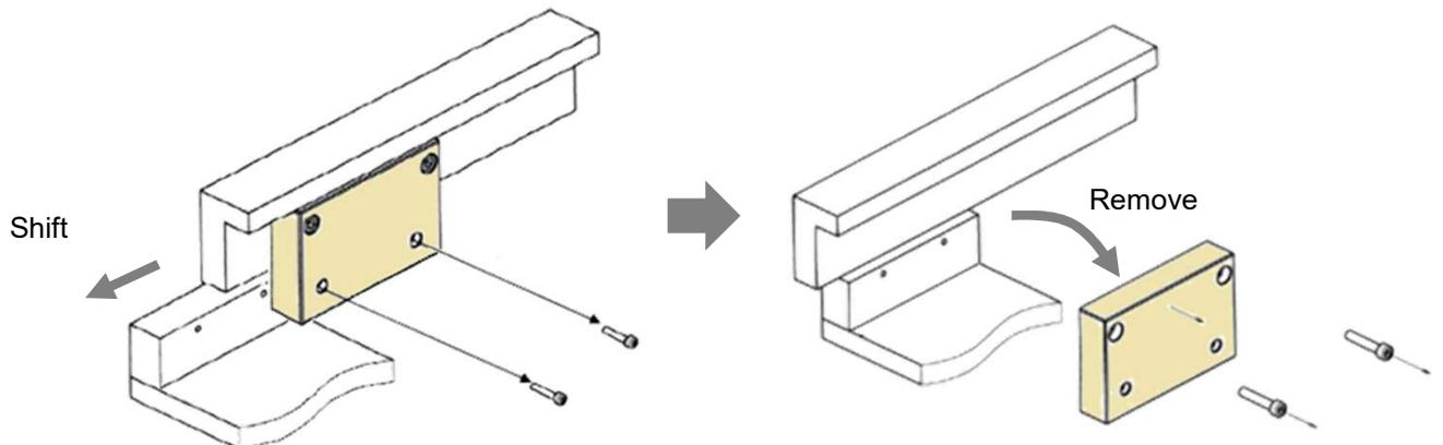
Check for interference and gap between positioning jig and head bracket
