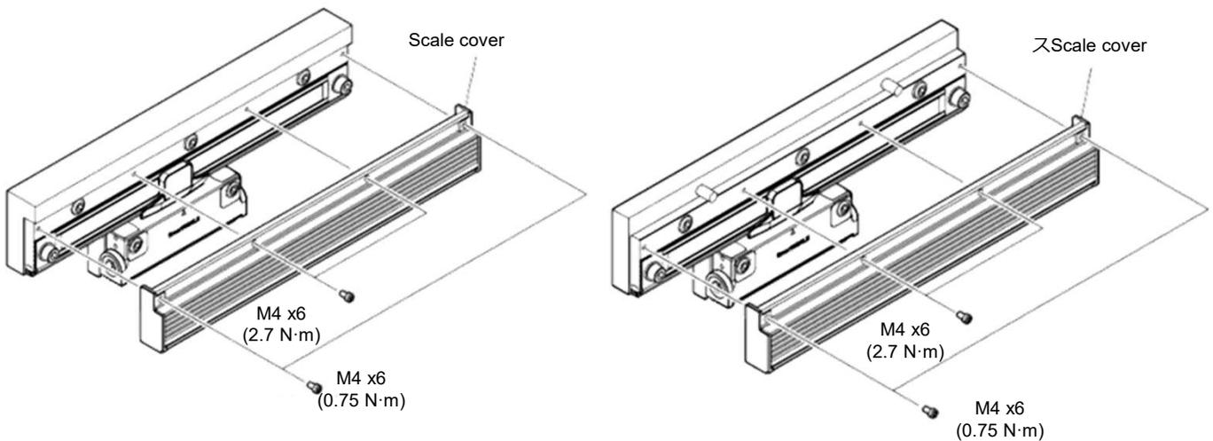
Pay attention to the screw tightening torque on both ends of the cover.
