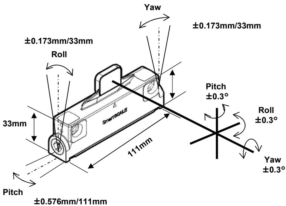
**Step ⑥: Mount the sensor head (Clearance adjustment)**
