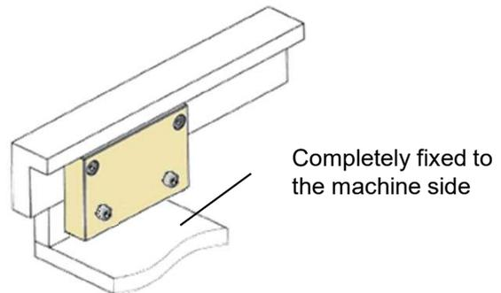
**Step ⑤: Removal of positioning jig**
