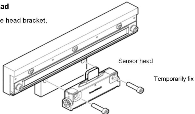
**Step ⑧: Mount the sensor head (Clearance adjustment)**
