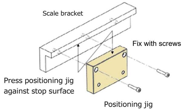
**Step ③: Installation of head bracket**
