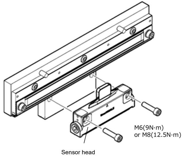
After adjusting with t0.185mm gauge, make sure **t=0.1mm gauge should enter the gap and t=0.25mm gauge should not enter the gap.**
