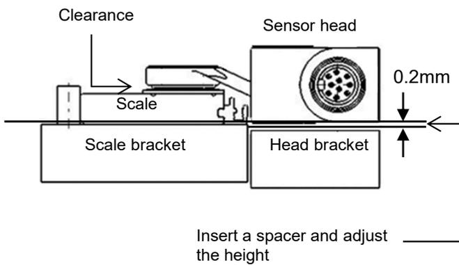
**When mounted on the top of the sensor head**
