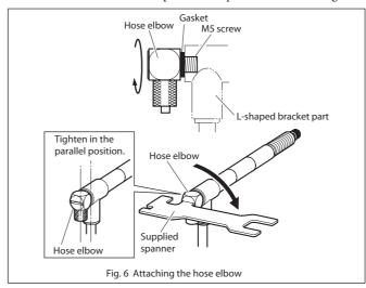
3. Attach the  $\phi 4$  mm air tube.
