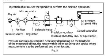
If the spindle ejection speed is too fast, an error may appear on the display the moment that the workpiece is touched. Excessive impact may dislodge the retainer inside the bearing, causing the measuring range to be reduced. In this case, use a speed controller as shown in Fig. 5 to adjust the spindle speed.
