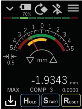
Reproduces the movement of a needle such as when using a lever gauge or dial gauge.
