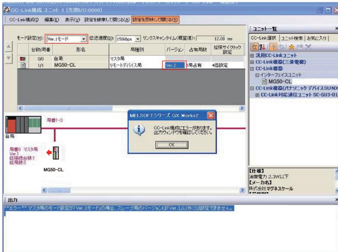
If the above error message is not displayed but communications are still not working (i.e., the RUN indicator on the MG50-CL does not light up), check to confirm that the switches for the baud rate, operating mode, and station number are all set correctly based on the parameters set for the master station.
