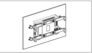
\* When using a commercially available stand that supports VESA75, pay attention to the length of the screws used to secure the display unit.
