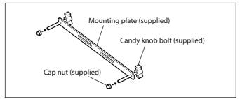
Insert the display unit through the mounting hole, and secure the mounting plates to the display unit with the supplied set screws.
