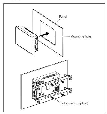
4. Tighten the candy knob bolts until they contact the panel to hold the display unit and mounting plates against the panel.
